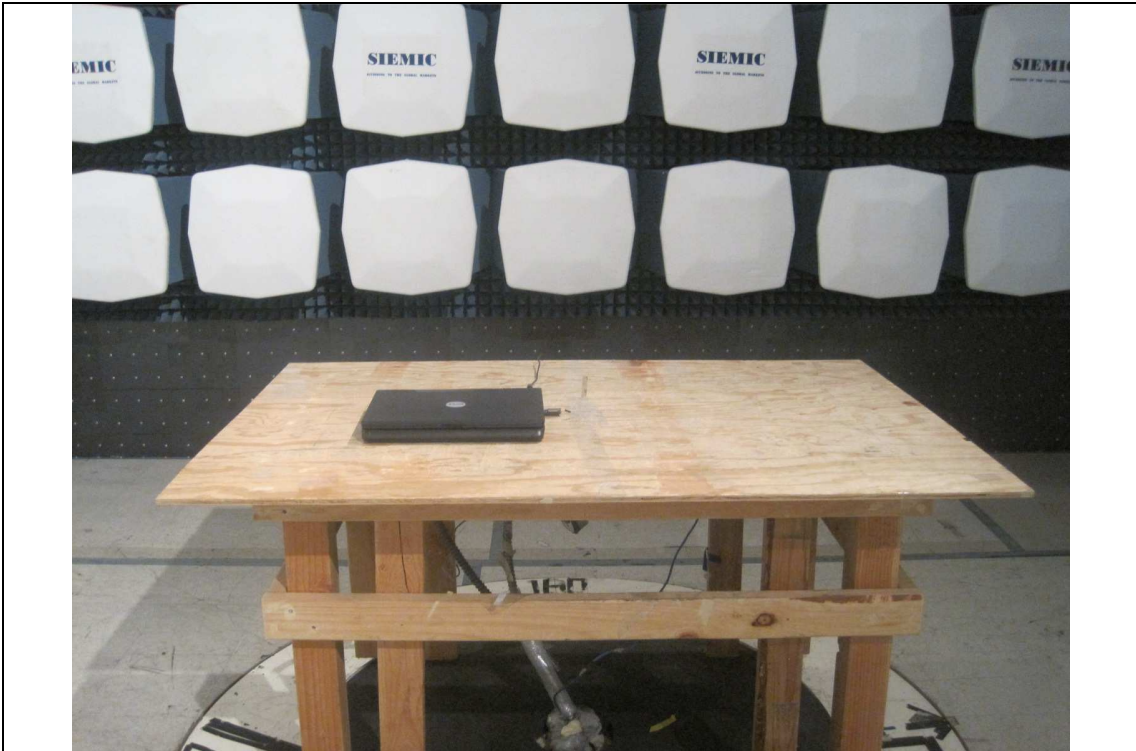
Radiated Emission Test Setup with patch antenna (30MHz – 1GHz) - Front View
