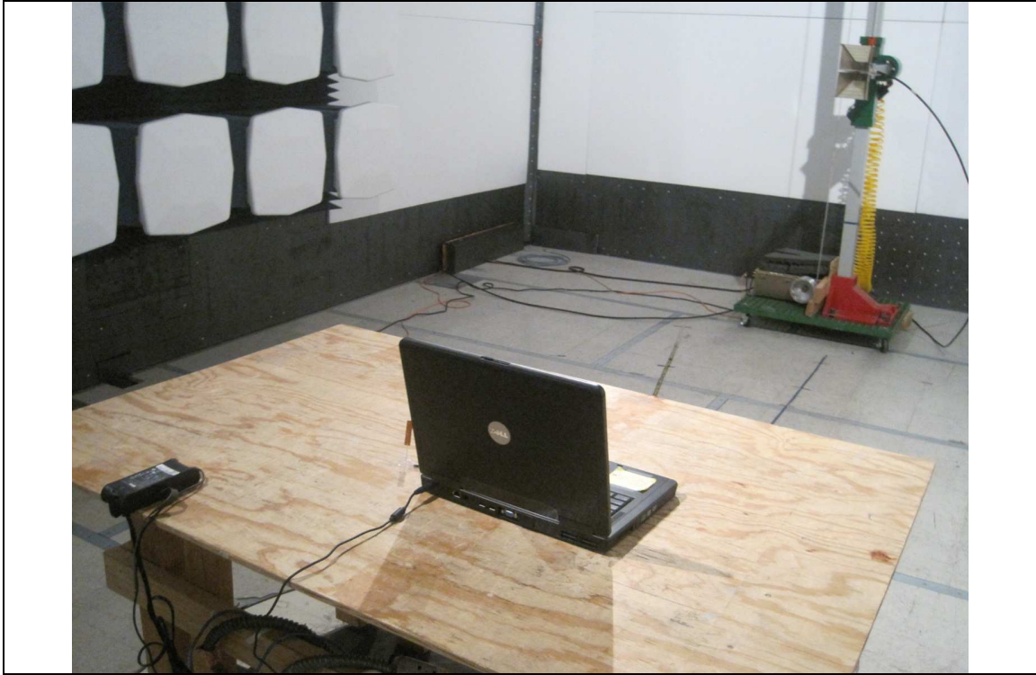
Radiated Emission Test Setup with patch antenna (Above 1GHz) - Front View
