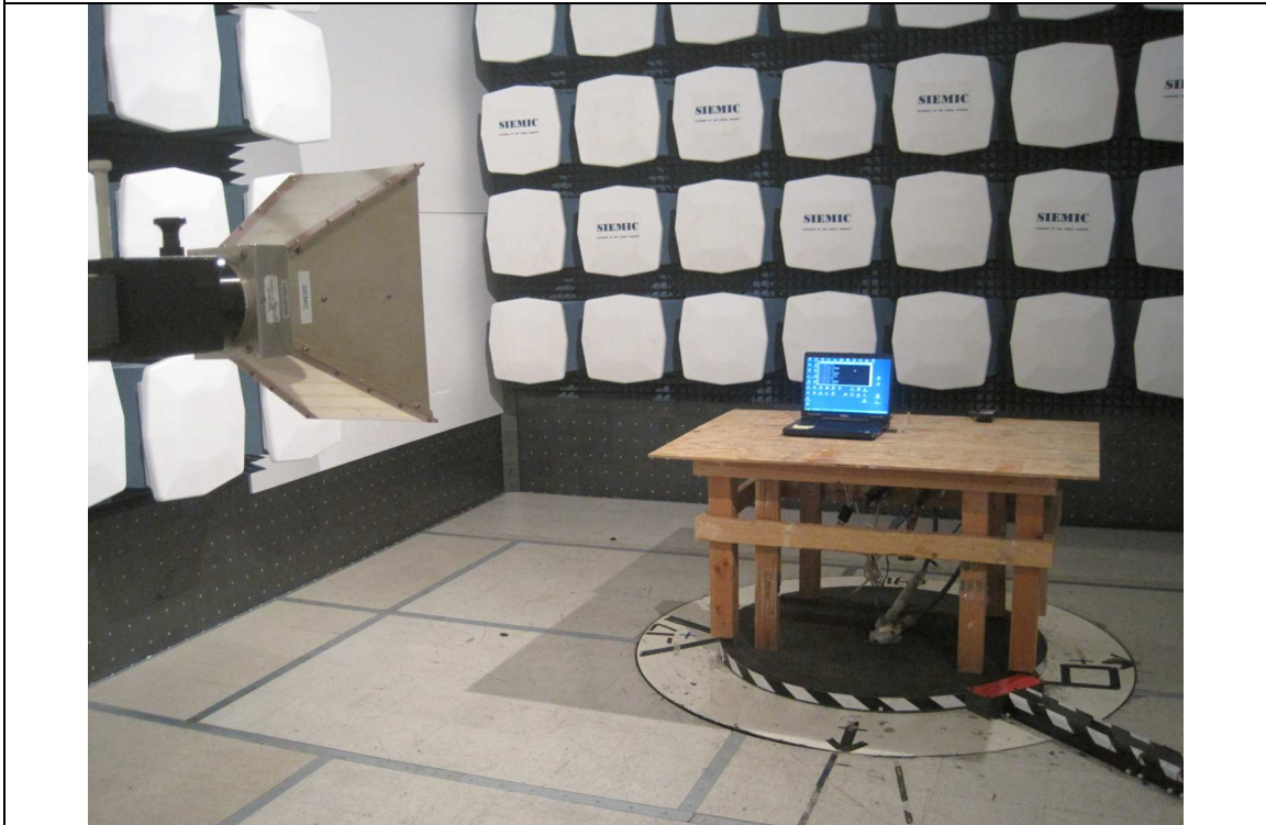
Radiated Emission Test Setup with patch antenna (above 1GHz) – Rear View
