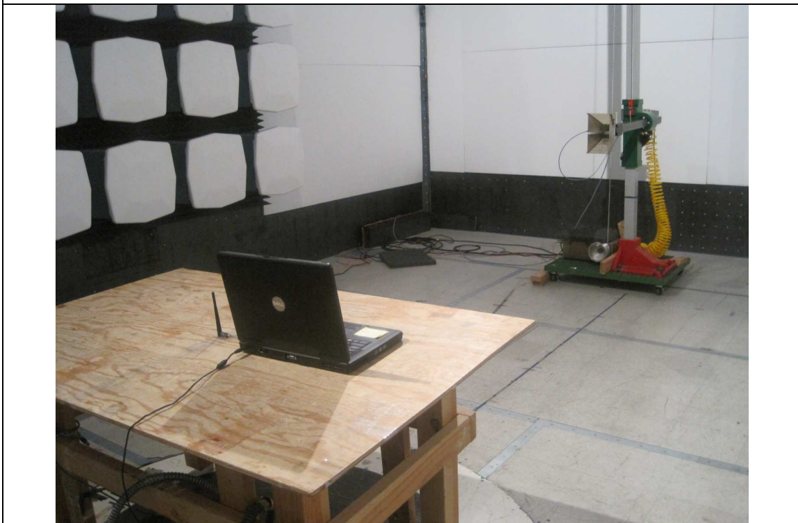
Radiated Emission Test Setup with dipole antenna (above 1GHz) – Rear View
