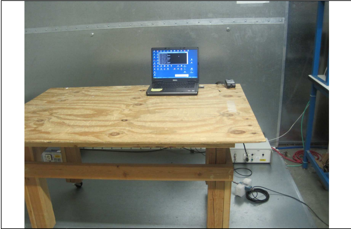
Conducted Emission Test Setup – Front View
