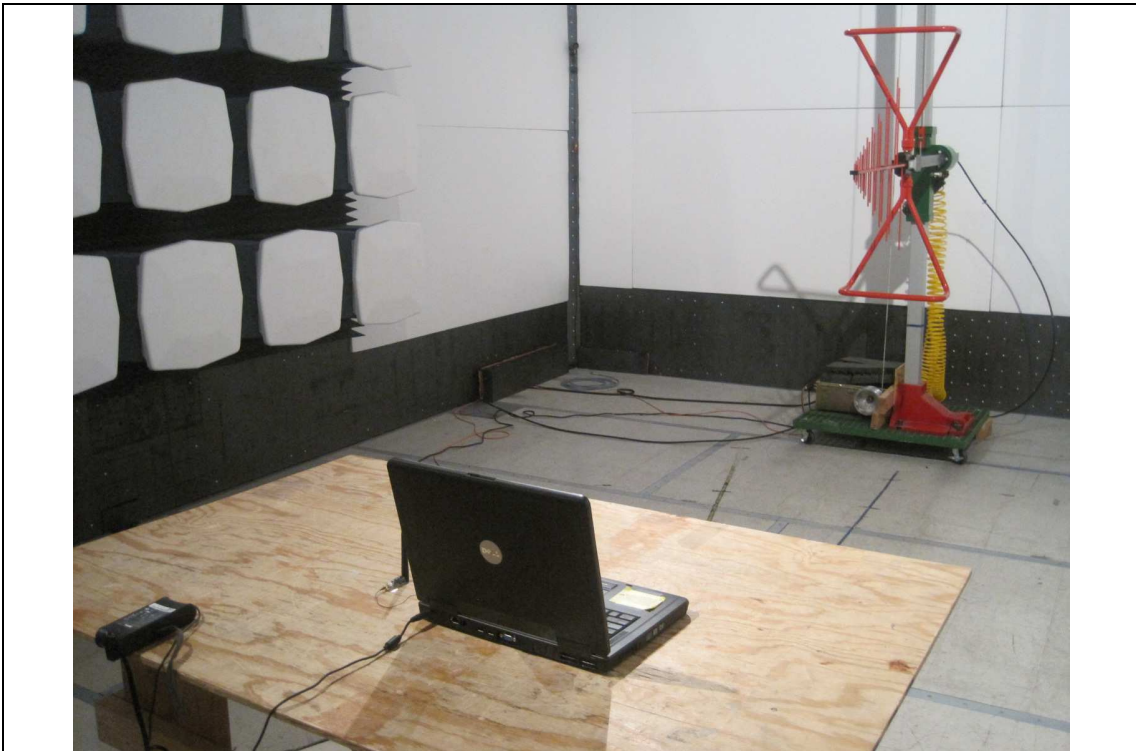
Radiated Emission Test Setup with dipole antenna (30MHz – 1GHz) - Front View
