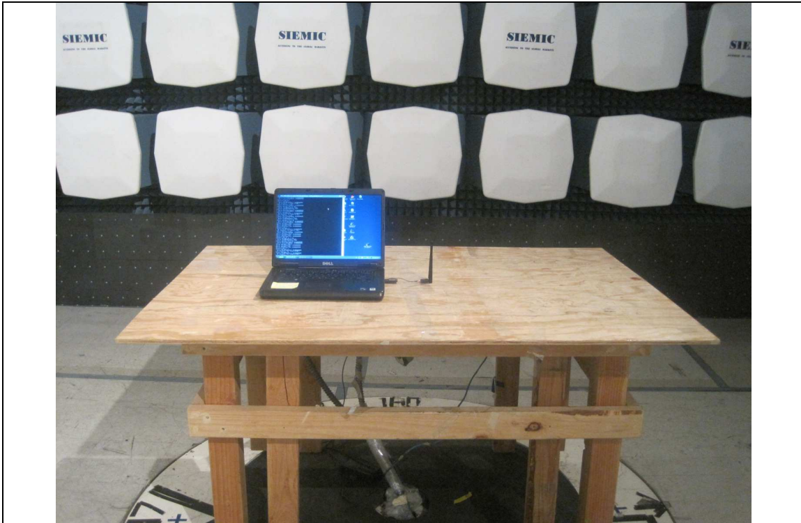
Radiated Emission Test Setup with dipole antenna (Above 1GHz) - Front View
