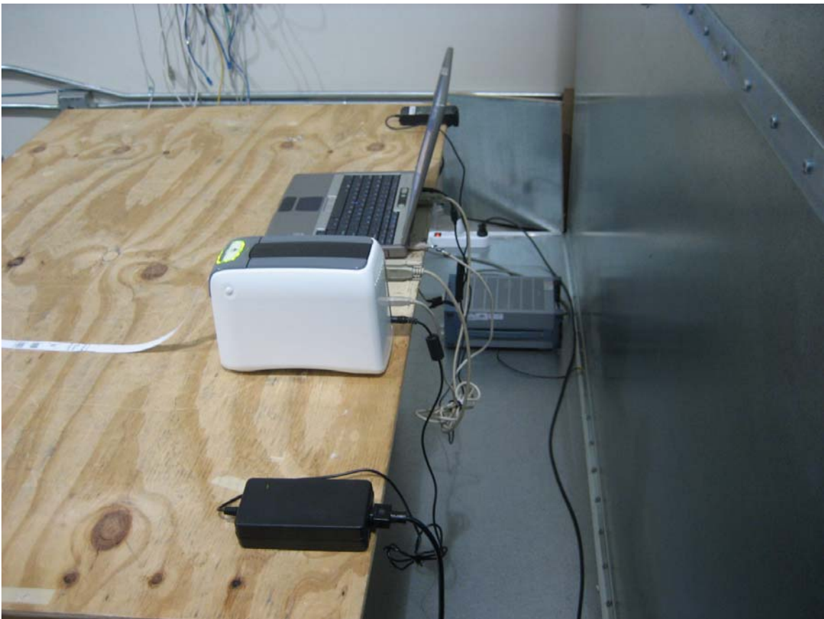
AC Line Conducted Emission Test Setup Rear View
