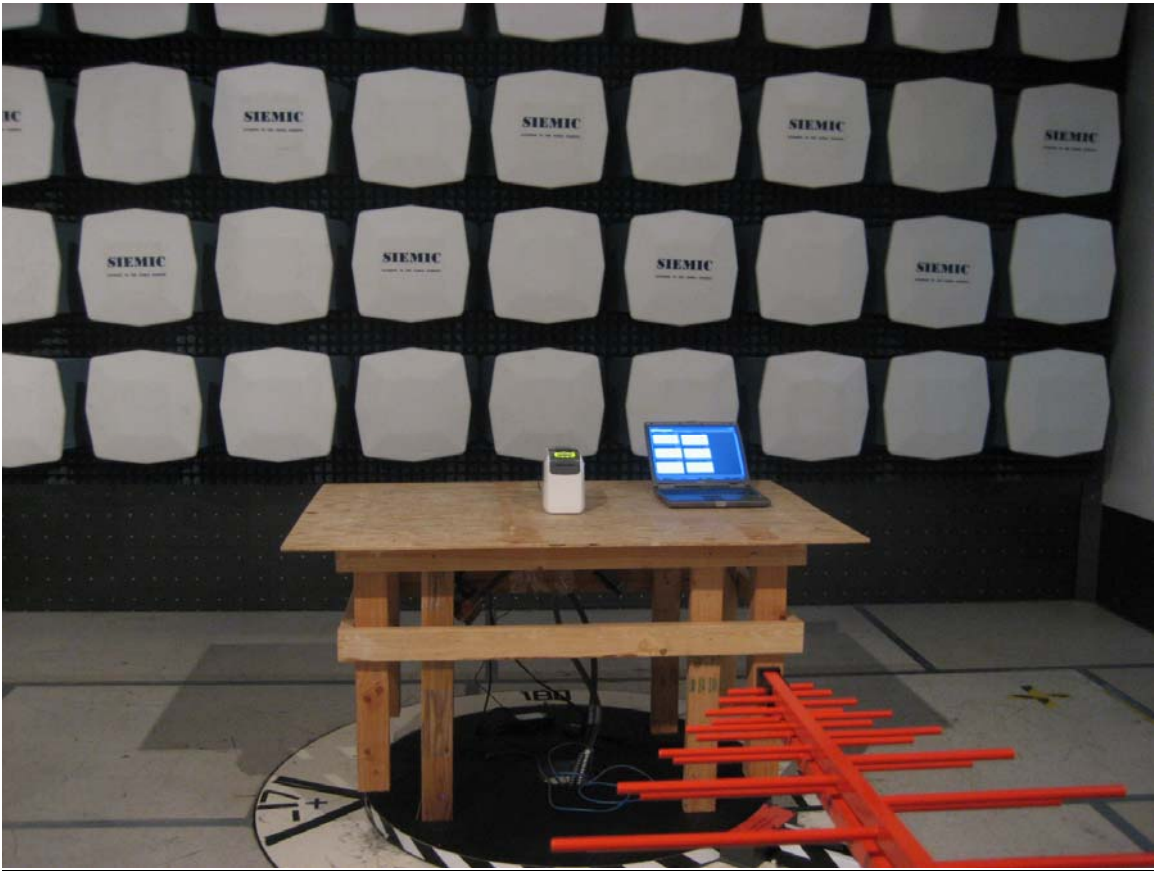
Radiated Emission Test Setup Front View (<1000MHz)
