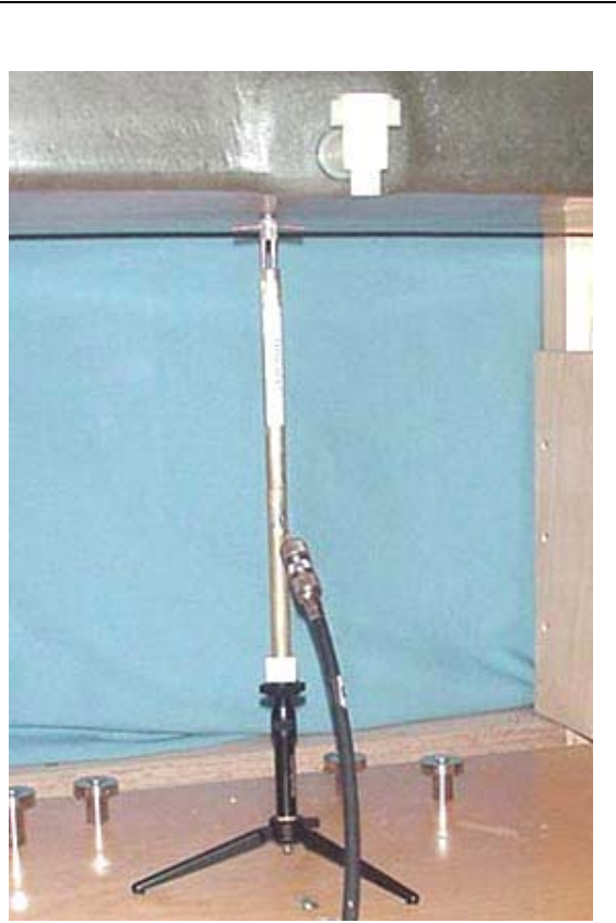
2450MHz Dipole Setup
