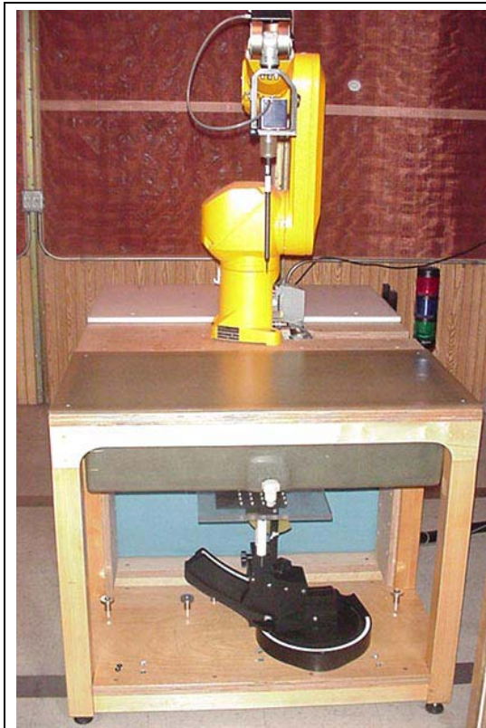
DASY4 SAR Measurement System & planar phantom
