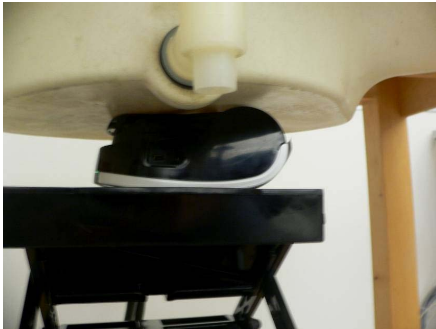
Model MZ220 back touching to the flat phantom with belt clip
