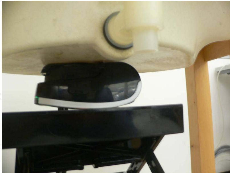
Model MZ320 back touching to the flat phantom with belt clip
