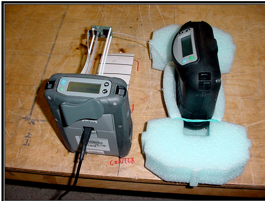
PHOTOGRAPH 14: CONDUCTED EMISSIONS REAR VIEW USING RW-420 CQ17252-1 ANTENNA
