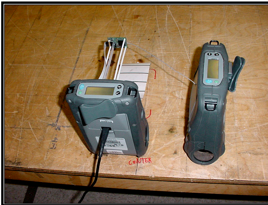
CONDUCTED EMISSIONS REAR VIEW USING QL-420 CQ17383-1 ANTENNA
