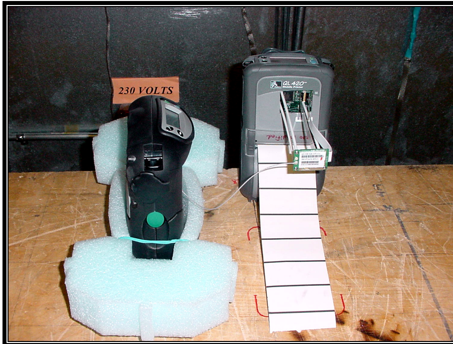
PHOTOGRAPH 13: CONDUCTED EMISSIONS FRONT VIEW USING RW-420 CQ17252-1 ANTENNA
