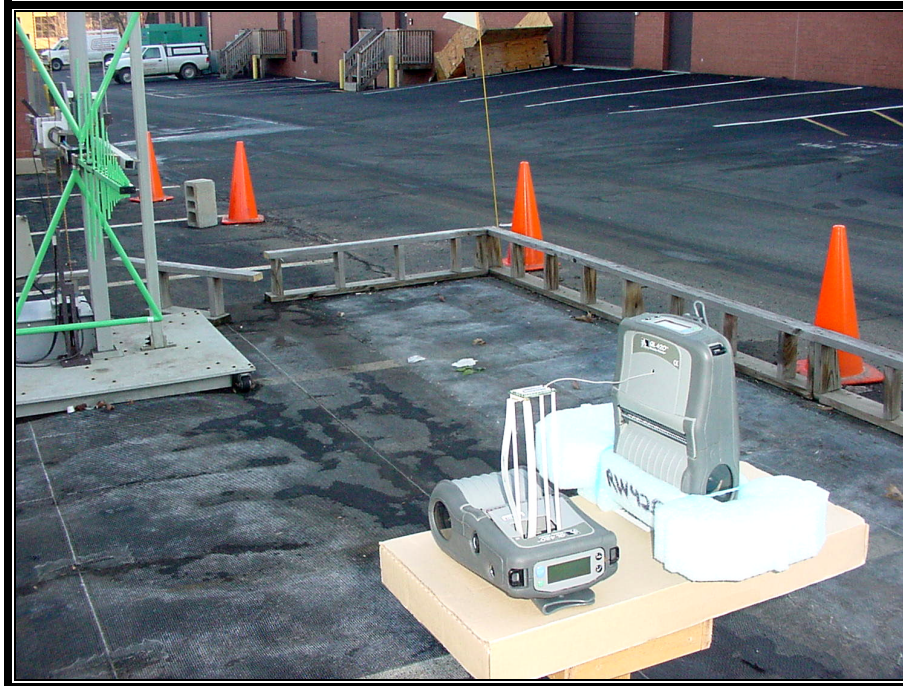
PHOTOGRAPH 5: RADIATED EMISSIONS FRONT VIEW USING QL-420 CQ17383-1 ANTENNA
