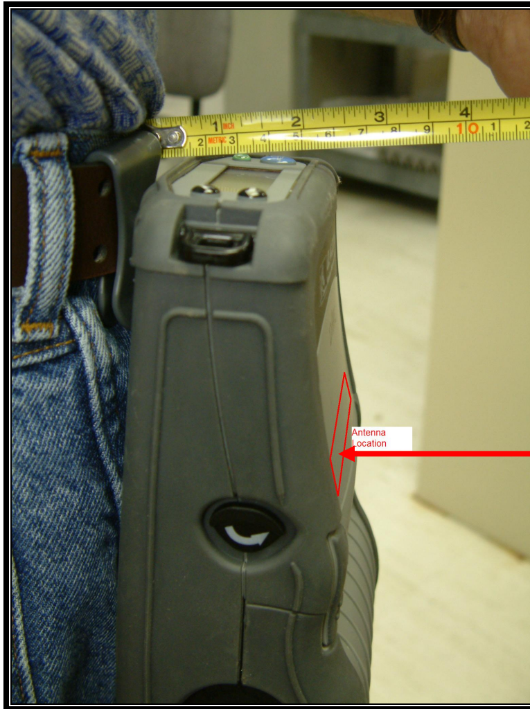
Photograph 3: QL320 side view showing separation distance between antenna and body
