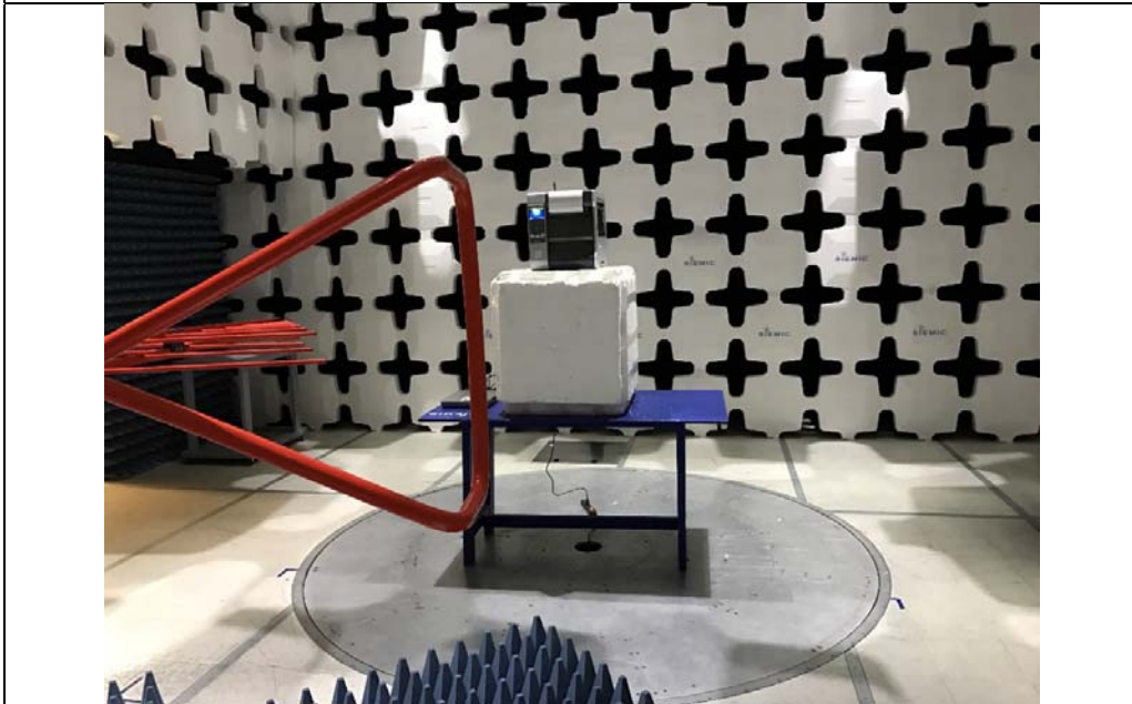
Radiated Emissions (<1GHz) – Rear View
