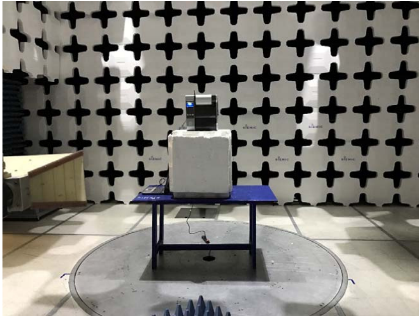
Radiated Emissions (>1GHz) – Front View
