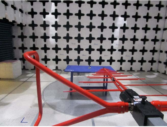
Radiated Emission Test setup (<1GHz) – Front View
