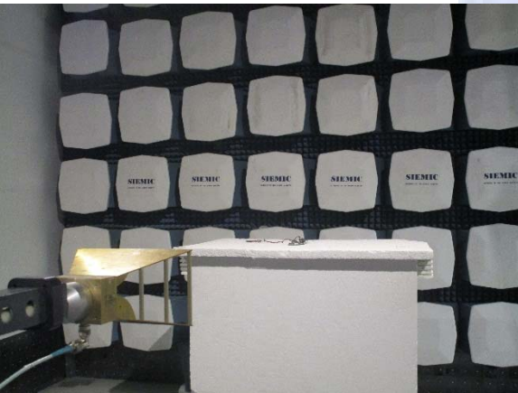
Radiated Emission Test setup (>1GHz) – Front View
