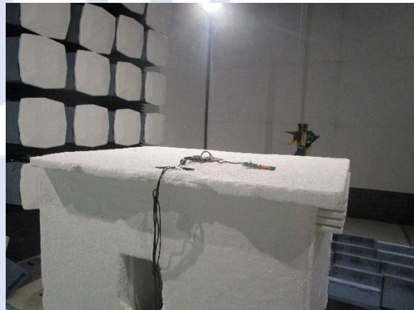
Radiated Emission Test setup (>1GHz) – Rear View
