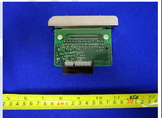
EUT Sub PCBA Parallel Port Board – Bottom View
