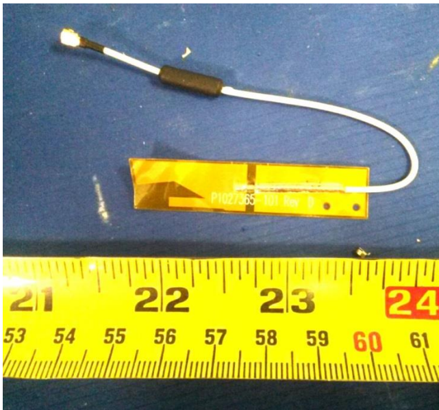
Antenna Top View
