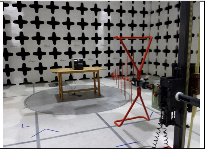
Radiated Emission below 1GHz – ZT410 (Rear)
