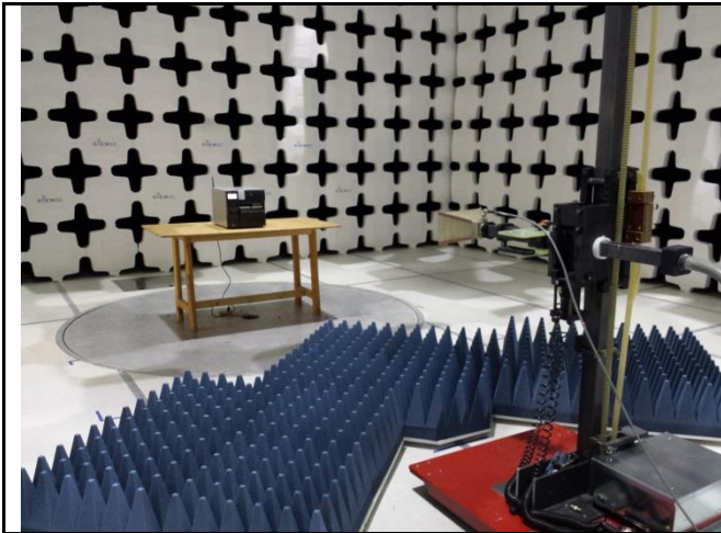
Radiated Emission above 1GHz – ZT420 (Front)
