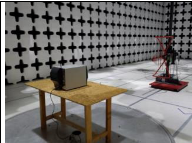
Radiated Emission below 1GHz – ZT410 (Front)
