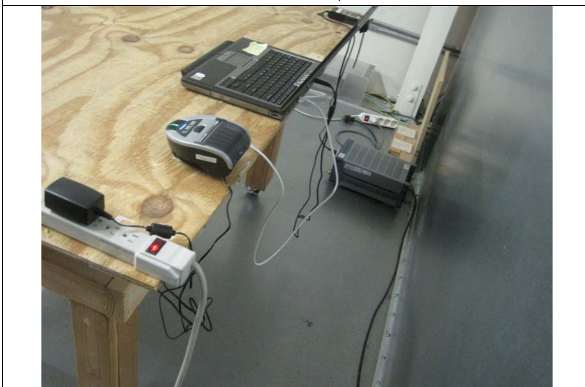
Conducted Emission Test Setup – Rear View
