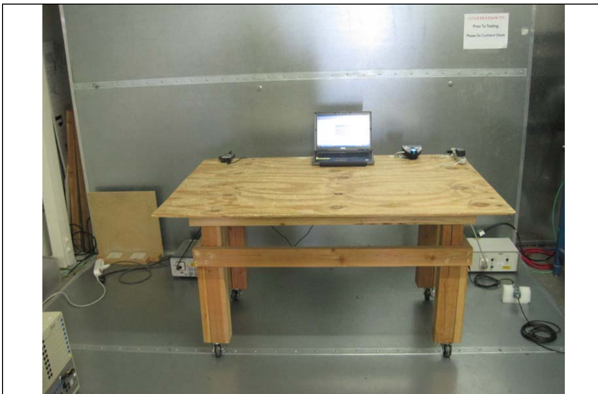
Conducted Emission Test Setup – Front View
