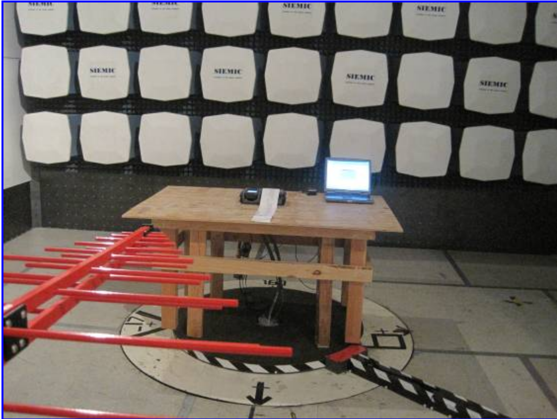
Radiated Emission Test Setup – Front View
