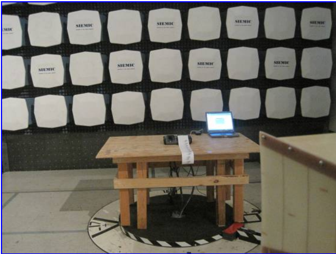
Radiated Emission Test Setup – Front View
