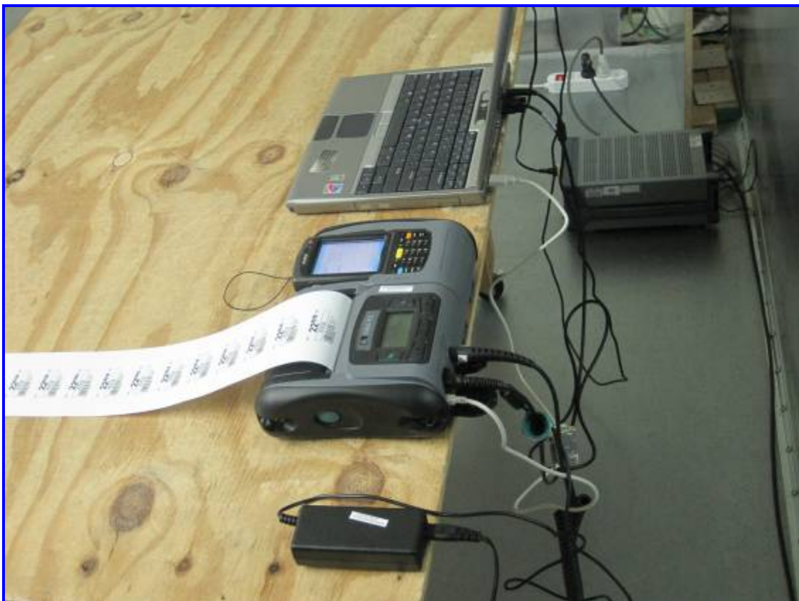
Conducted Emission Test Setup – Rear View
