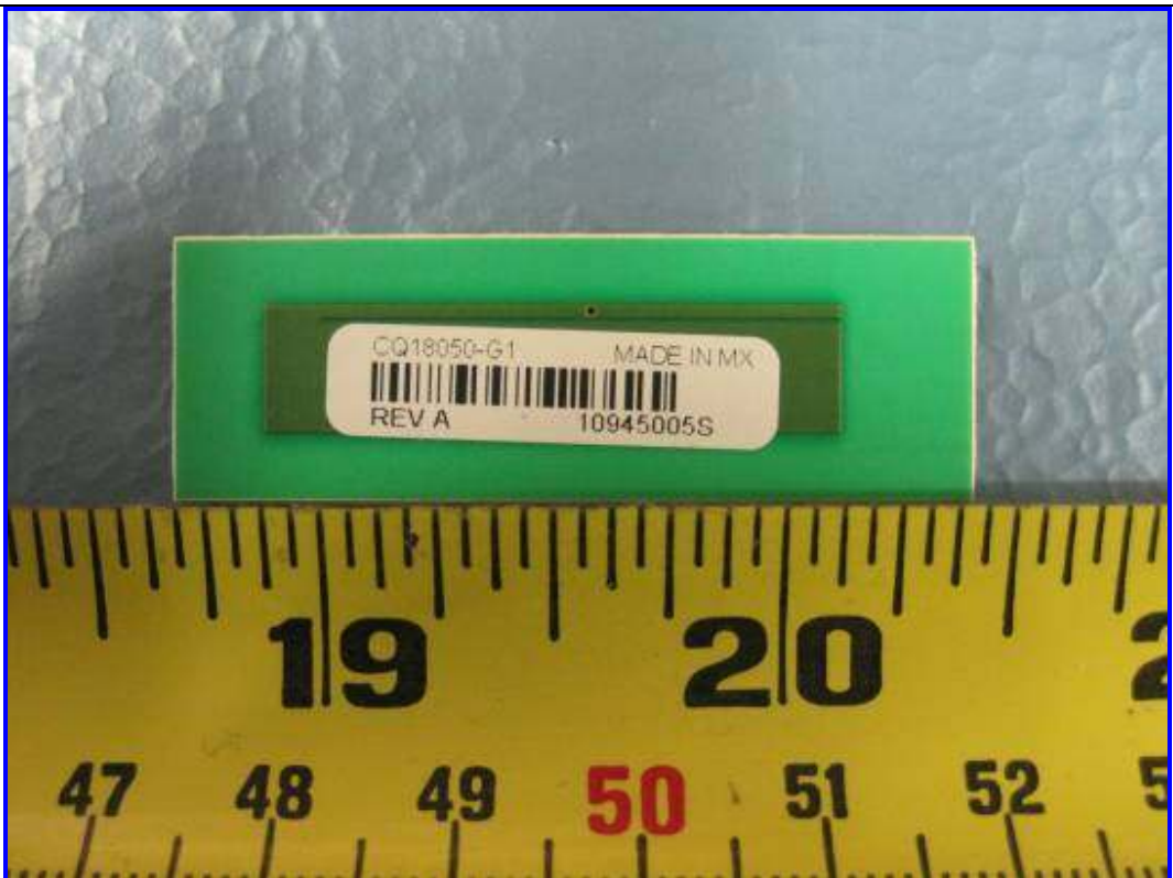
EUT: Antenna Board Solder View
