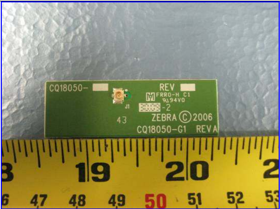
EUT: Antenna Board Component View
