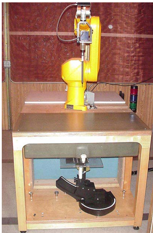
DASY4 SAR Measurement System with planar phantom
