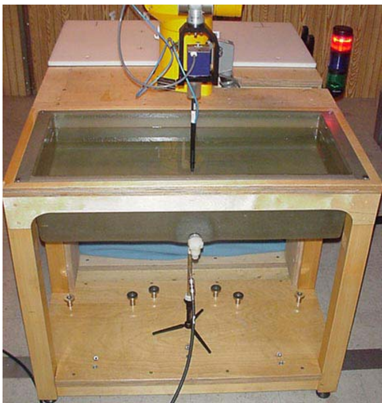
DASY4 SAR Measurement System with planar phantom and validation dipole
