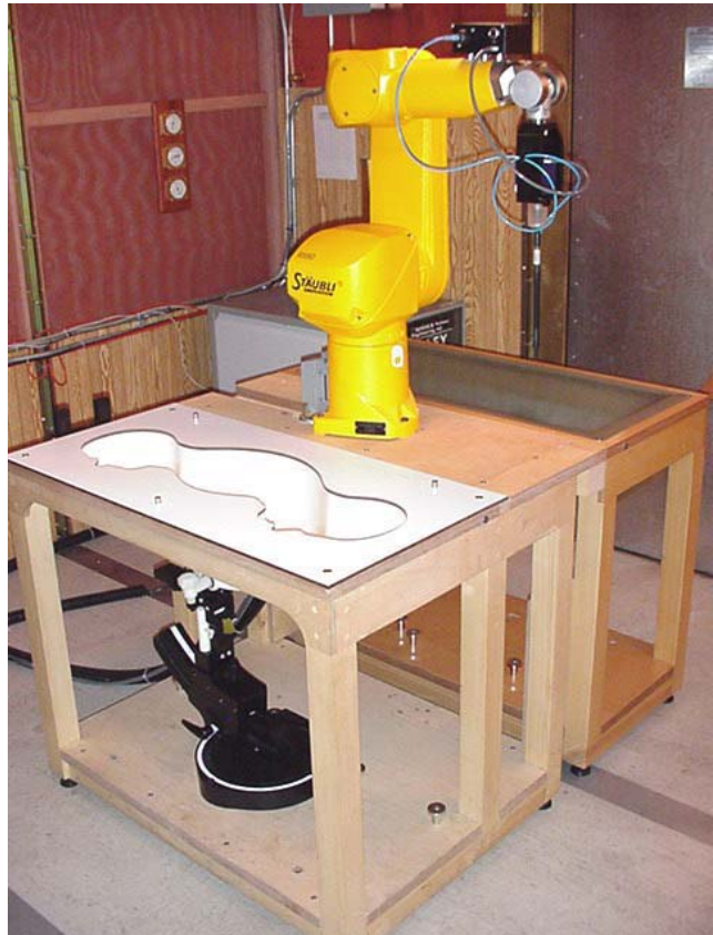
DASY4 SAR Measurement System with SAM phantom
