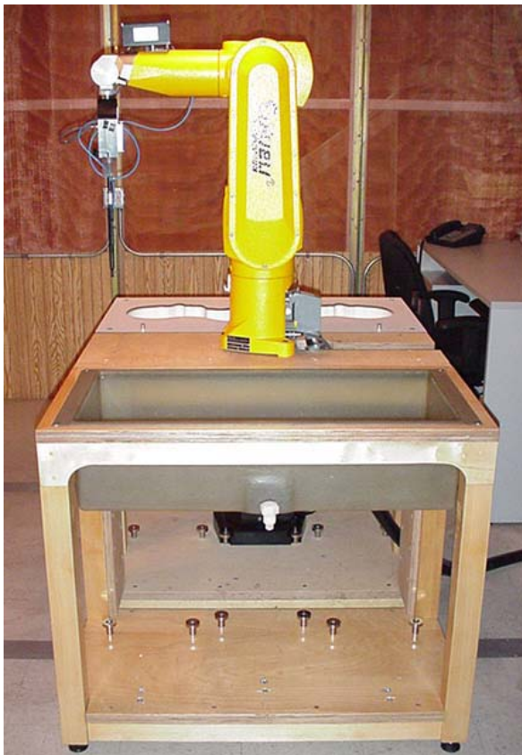
DASY4 SAR Measurement System with planar phantom
