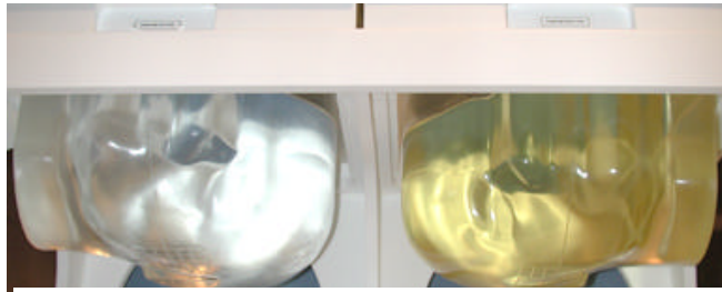
Figure 7.1 Left and Right SAM Phantom shells
