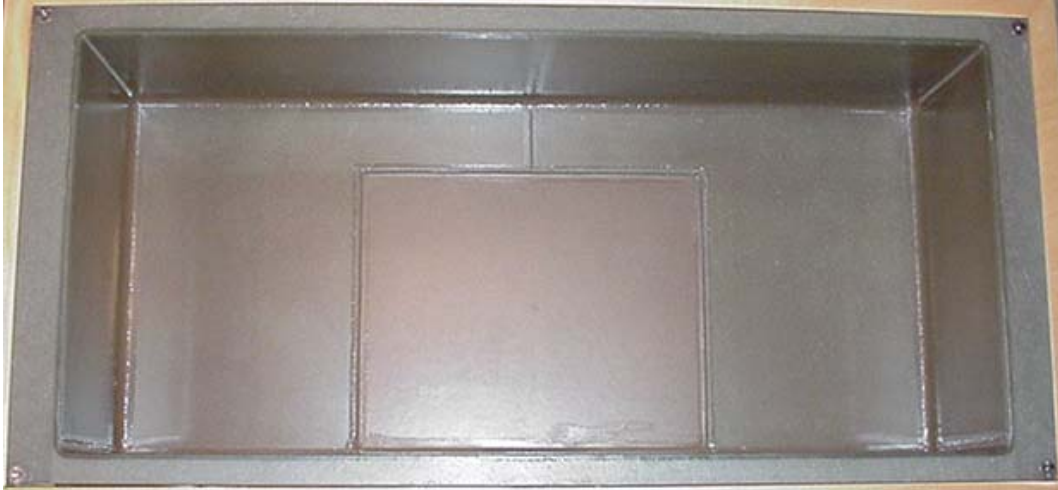
Fiberglass Planar Phantom - Top View
