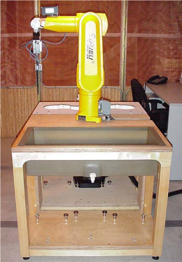
DASY4 SAR Measurement System with planar phantom
