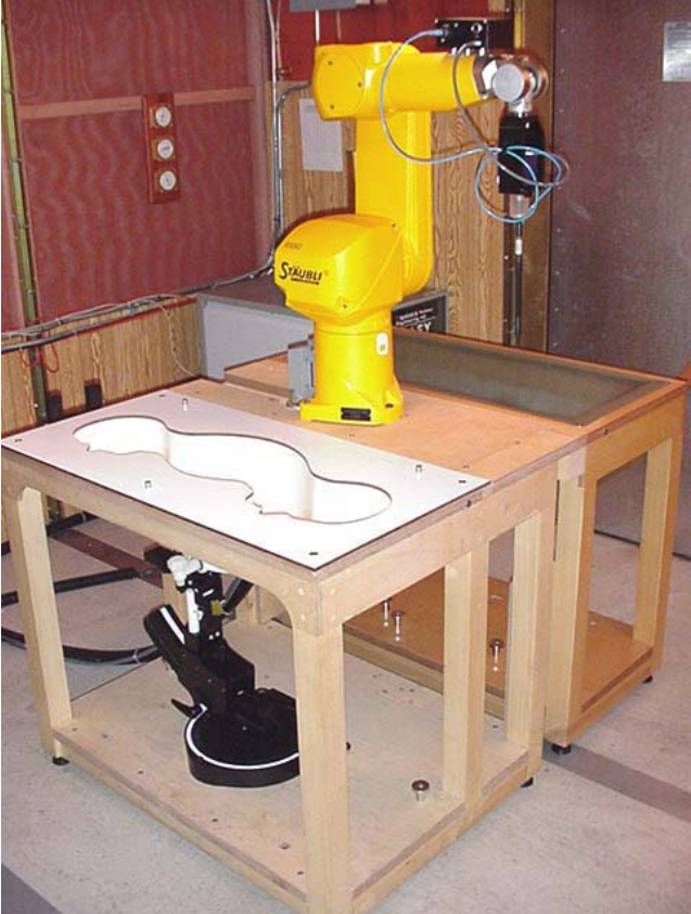
DASY4 SAR Measurement System with SAM phantom
