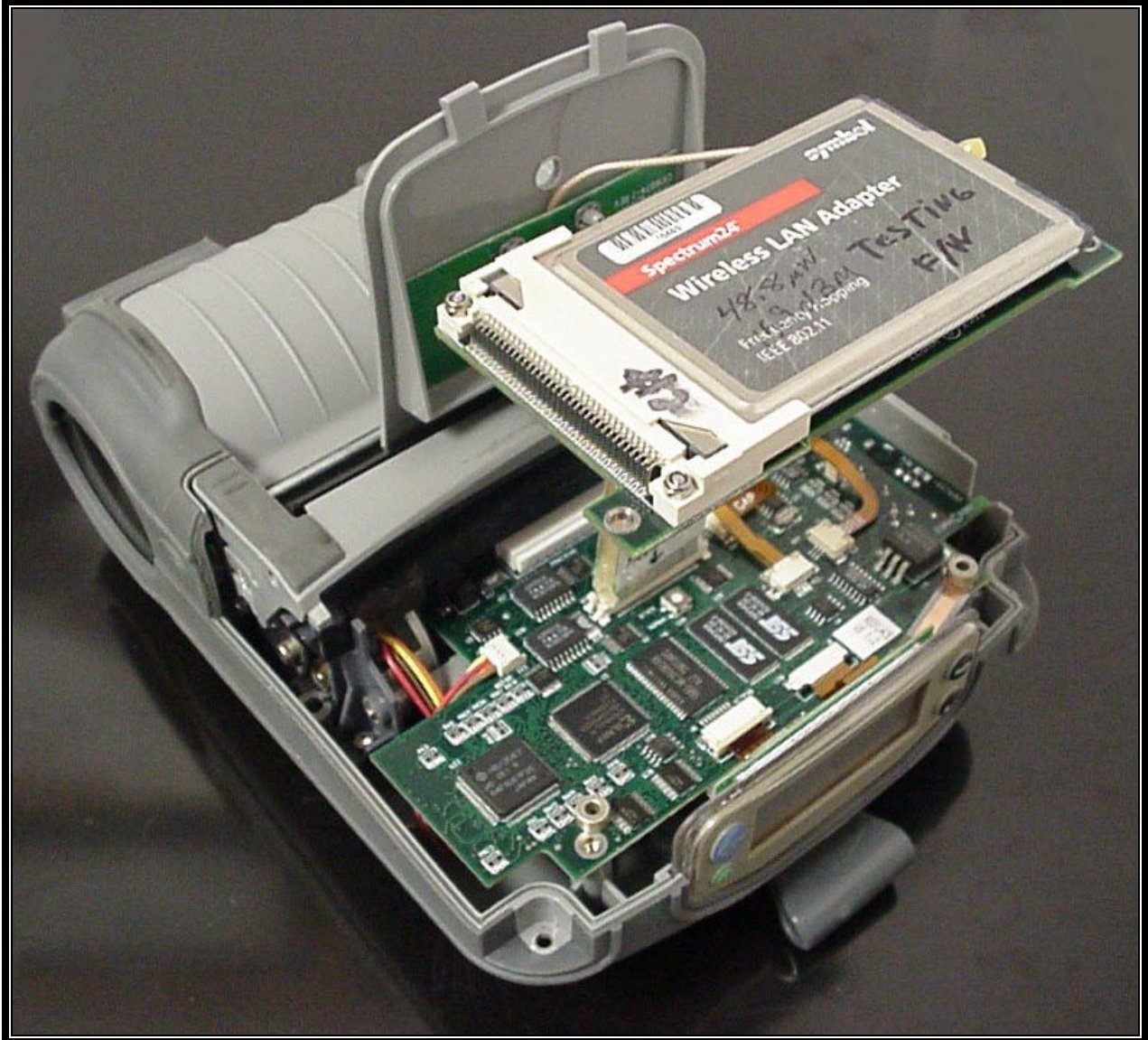
PHOTOGRAPH 3: VIEW OF MODULE MOUNTED EXTERNALLY FOR RADIATED TESTING
