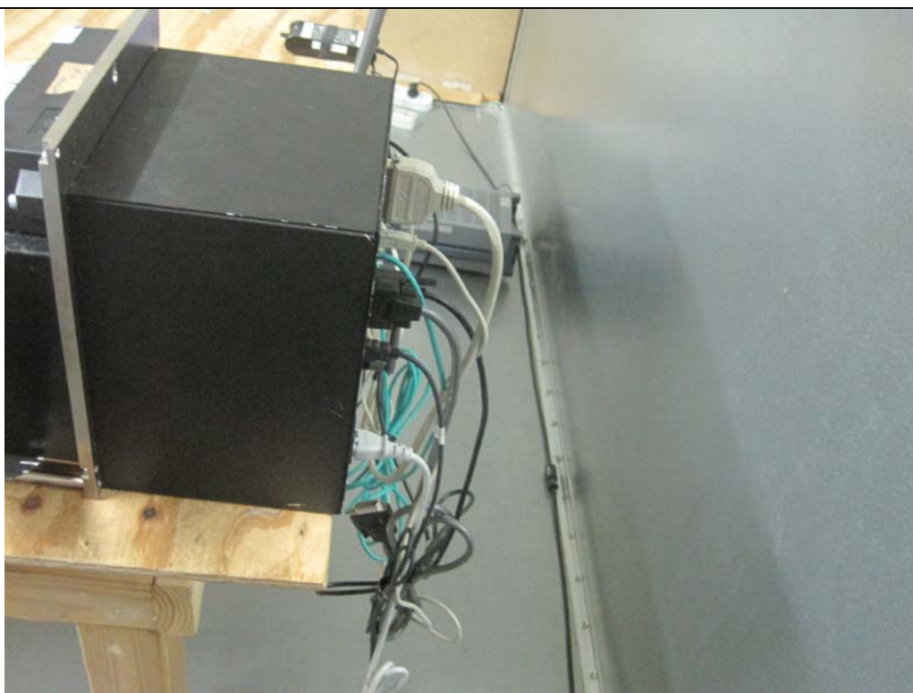
Conducted Emission Test Setup – Rear View
