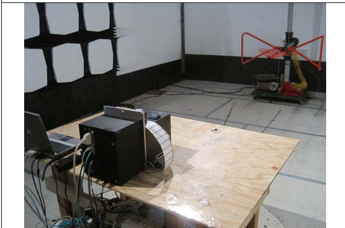
Radiated Emission Test Setup (below 1GHz) - Rear View
