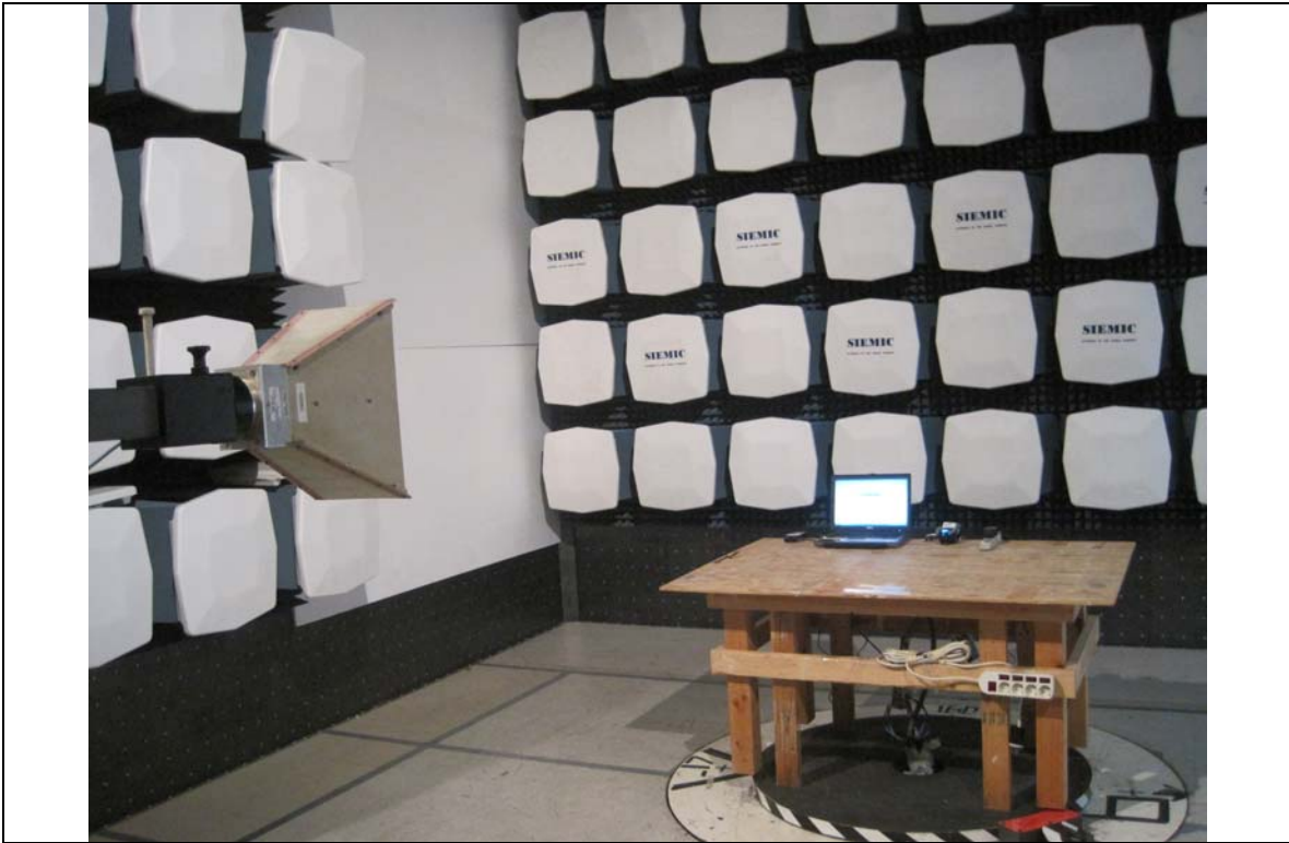
Radiated Emission Test Setup (above 1GHz) - Front View
