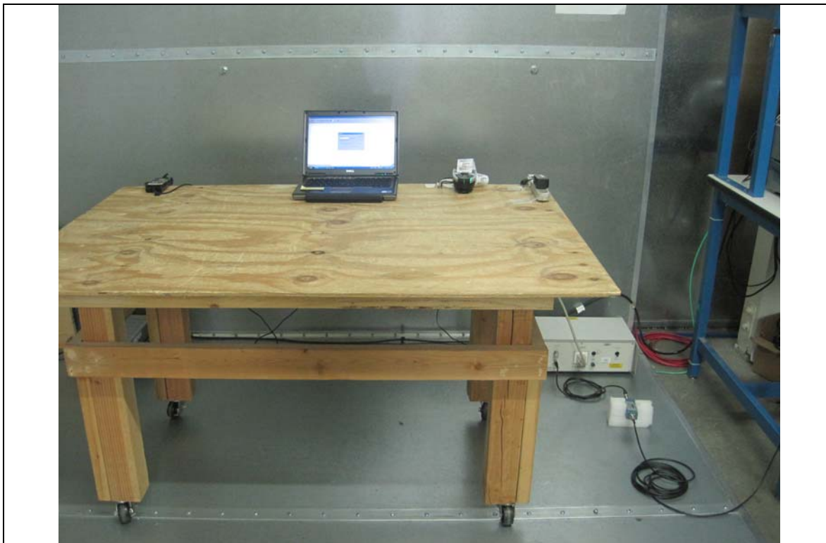
Conducted Emission Test Setup – Front View
