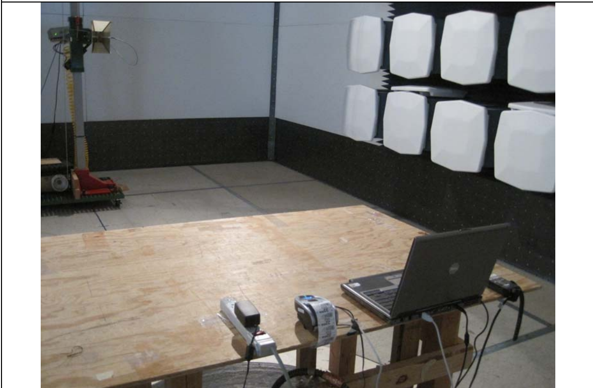
Radiated Emission Test Setup (above 1GHz) - Rear View
