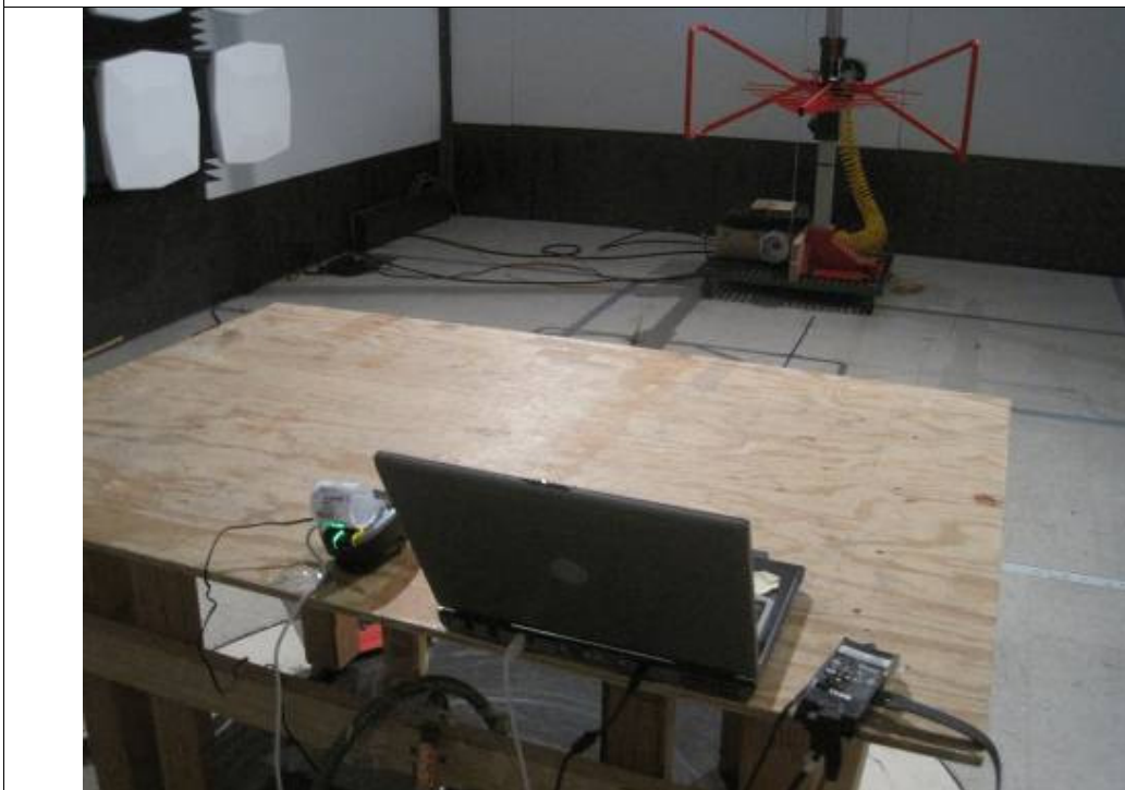
Radiated Emission Test Setup (above 1GHz) – Rear View
