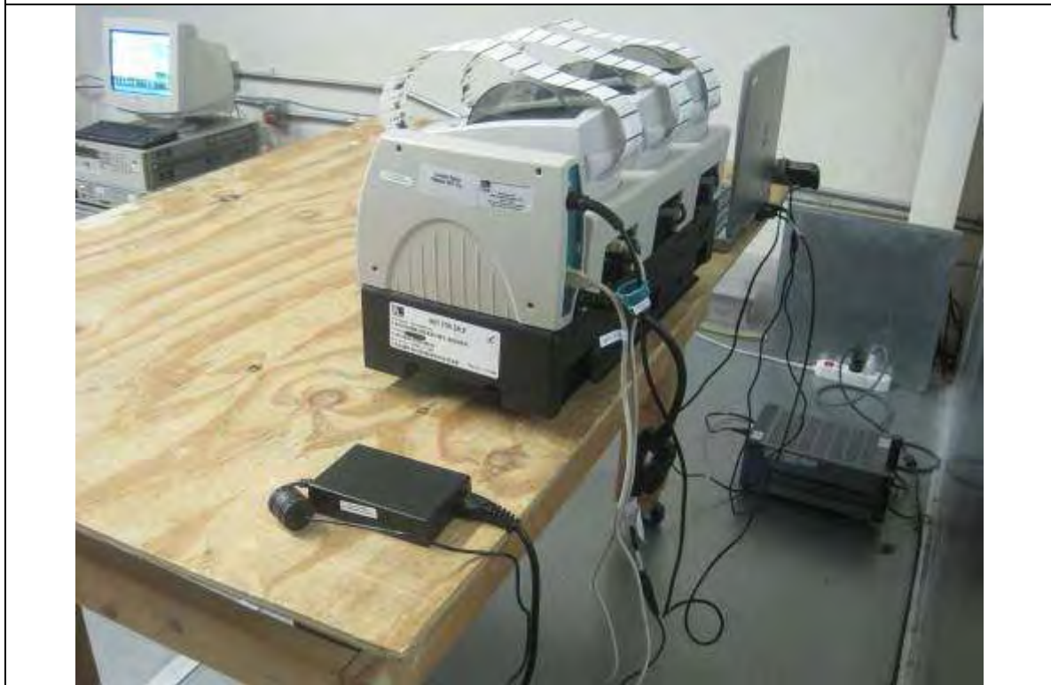
Conducted Emission Test Setup – Rear View
