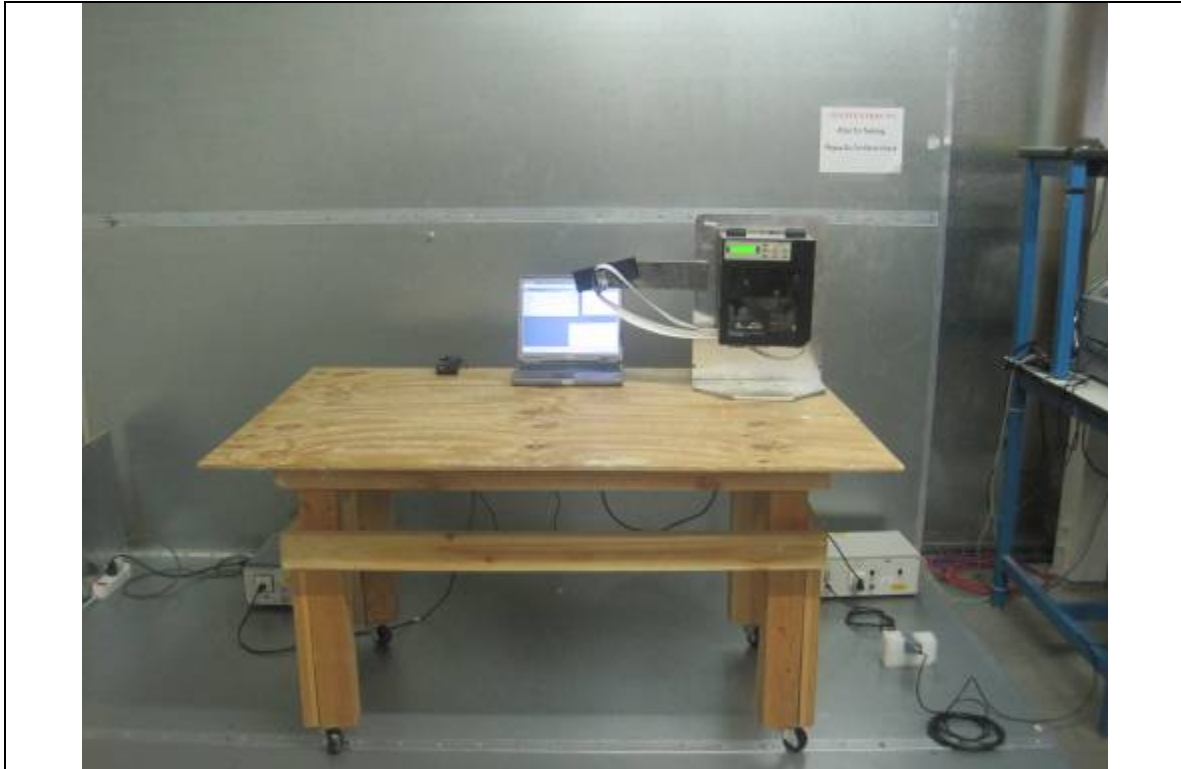
Conducted Emission Test Setup – Front View
