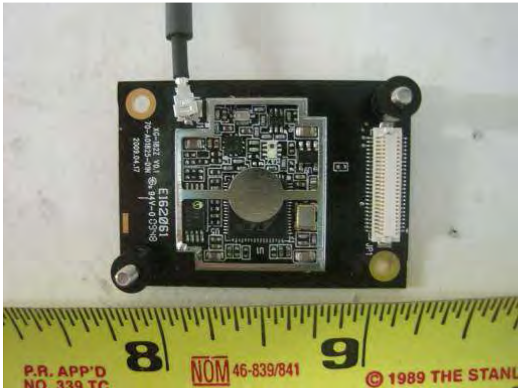
Radio Board shielding off View
