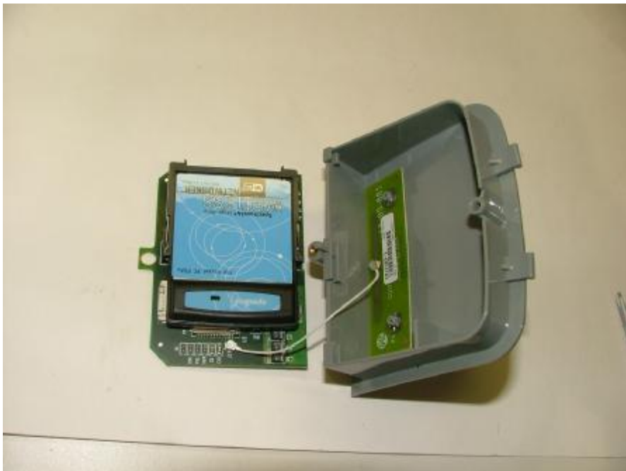
RF Carrier Board with H9PLA4137 and I28MD-BTC2TY4 Installed
