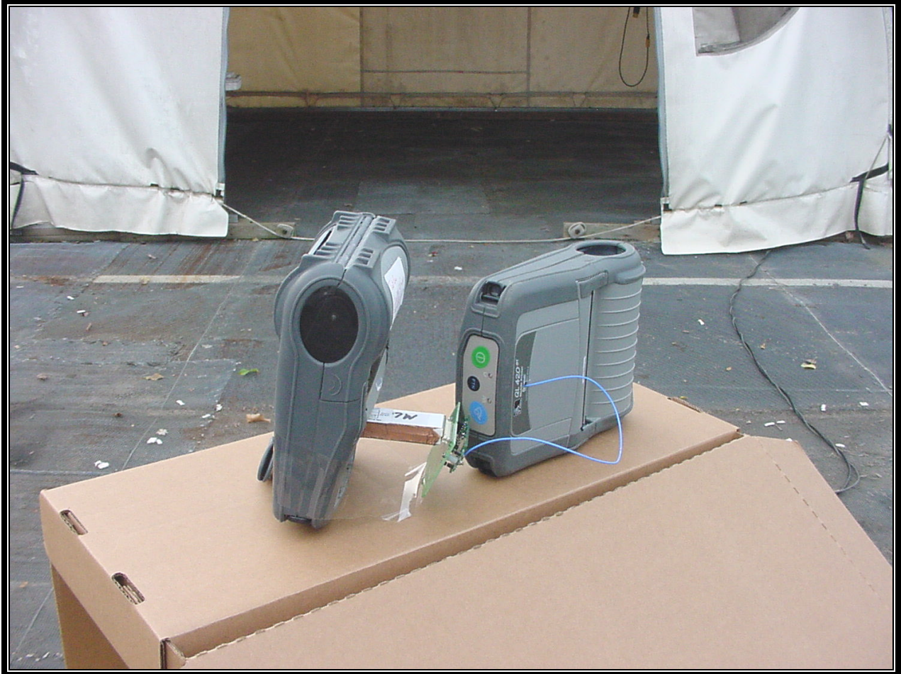
PHOTOGRAPH 12: RADIATED EMISSION FRONT VIEW, WORST CASE CONFIGURATION QL FAMILY (CC16203-2) ANTENNA
