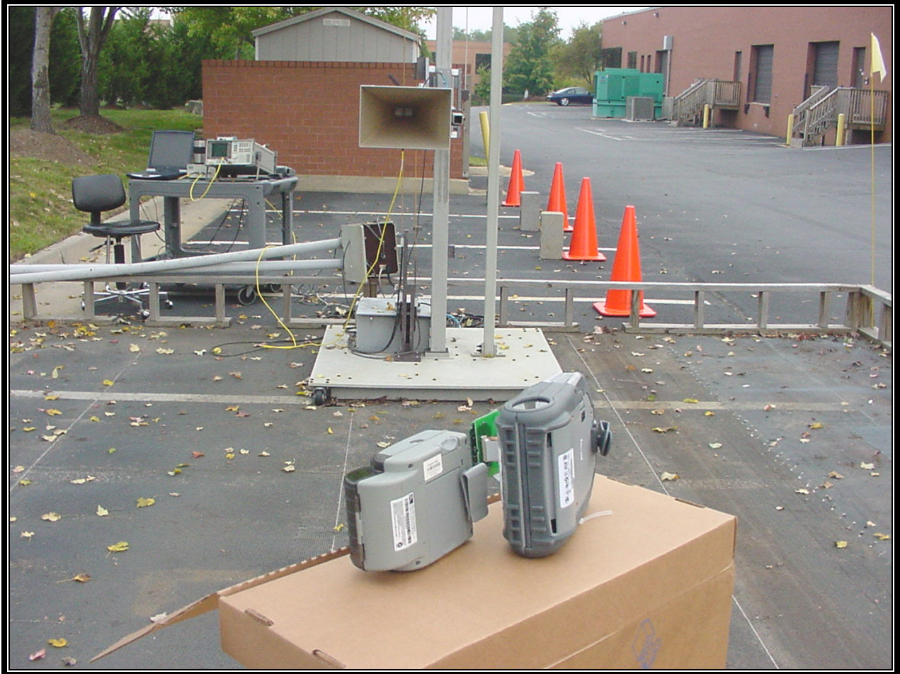
PHOTOGRAPH 11: RADIATED EMISSION REAR VIEW, WORST CASE CONFIGURATION CAMEO 3 (CQ15352-1) ANTENNA
