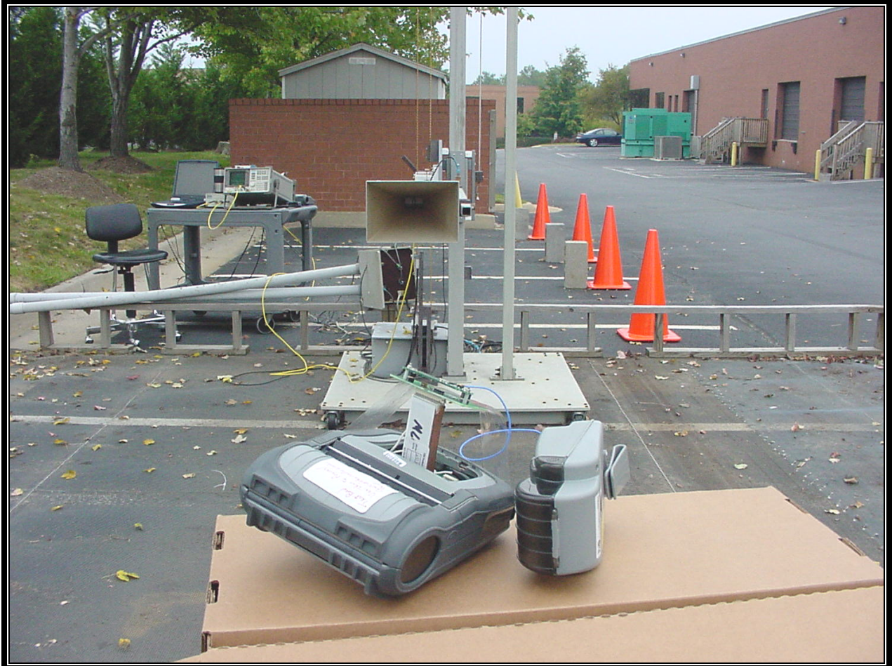
PHOTOGRAPH 9: RADIATED EMISSION REAR VIEW, WORST CASE CONFIGURATION CAMEO 2 (CQ15731-1) ANTENNA
