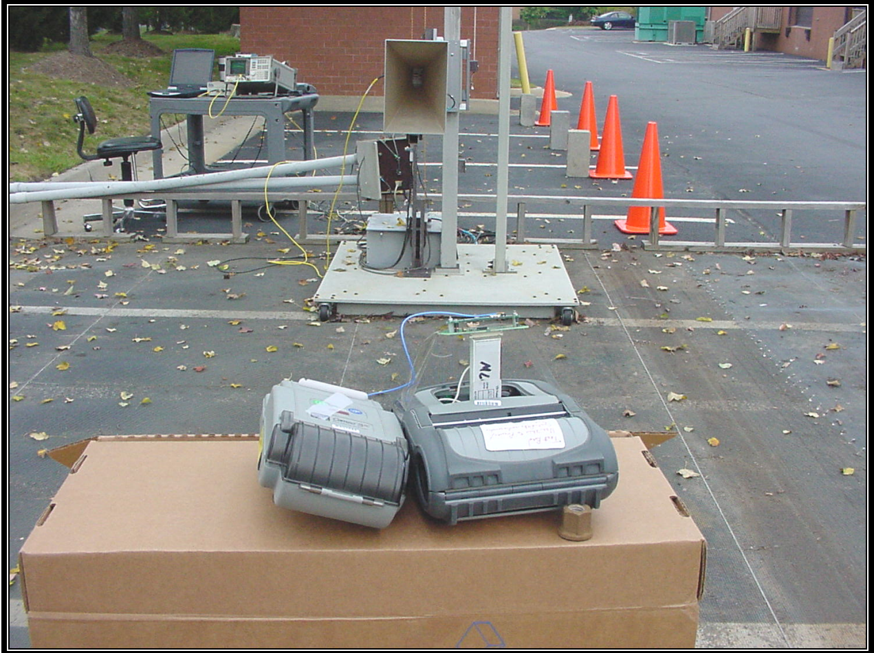
PHOTOGRAPH 5: RADIATED EMISSION REAR VIEW; WORST CASE CONFIGURATION CAMEO 3 SC (CQ16142-1) ANTENNA
