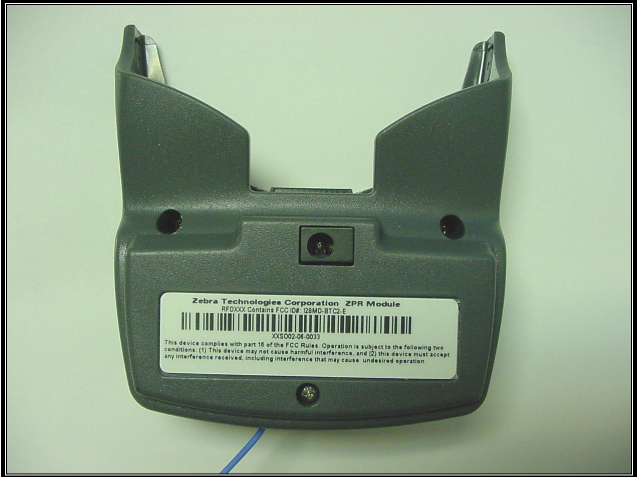
PHOTOGRAPH 31: REAR VIEW ZPR POD ANTENNA INSTALLED IN TYPICAL HOST
