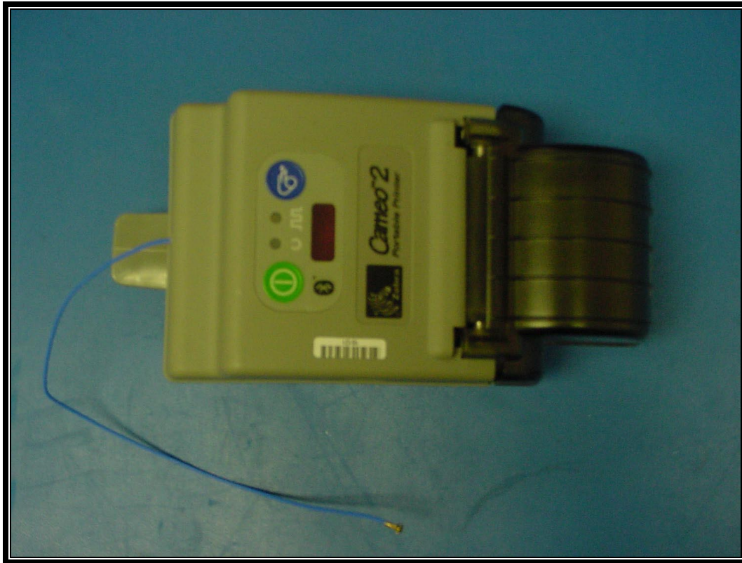
PHOTOGRAPH 18: TOP VIEW CAMEO 2 ANTENNA INSTALLED IN TYPICAL HOST
