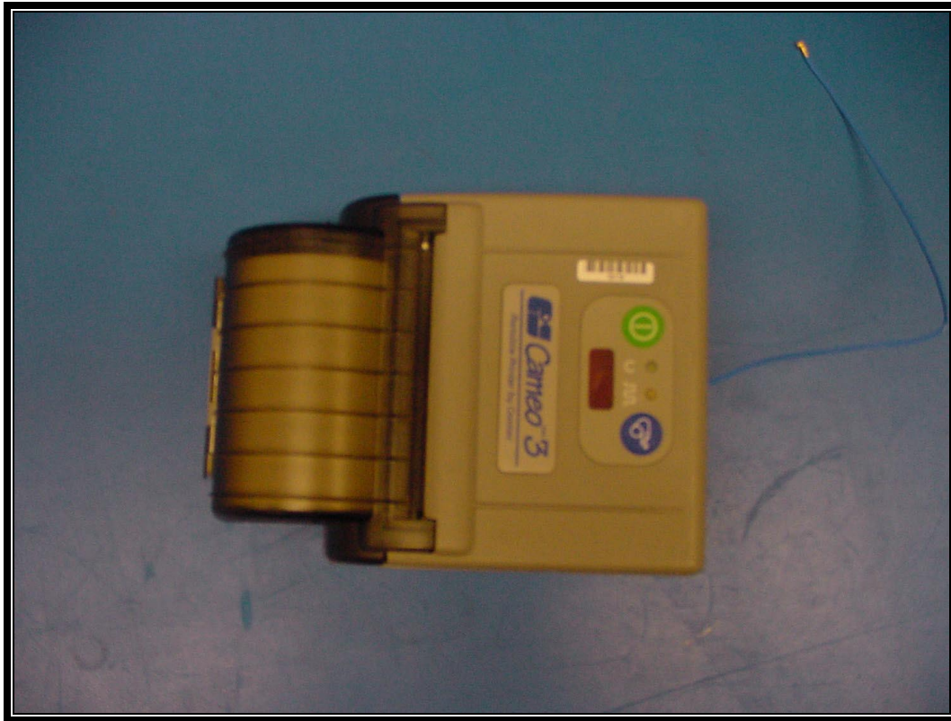
PHOTOGRAPH 22: FRONT VIEW CAMEO 3 SC ANTENNA INSTALLED IN TYPICAL HOST
