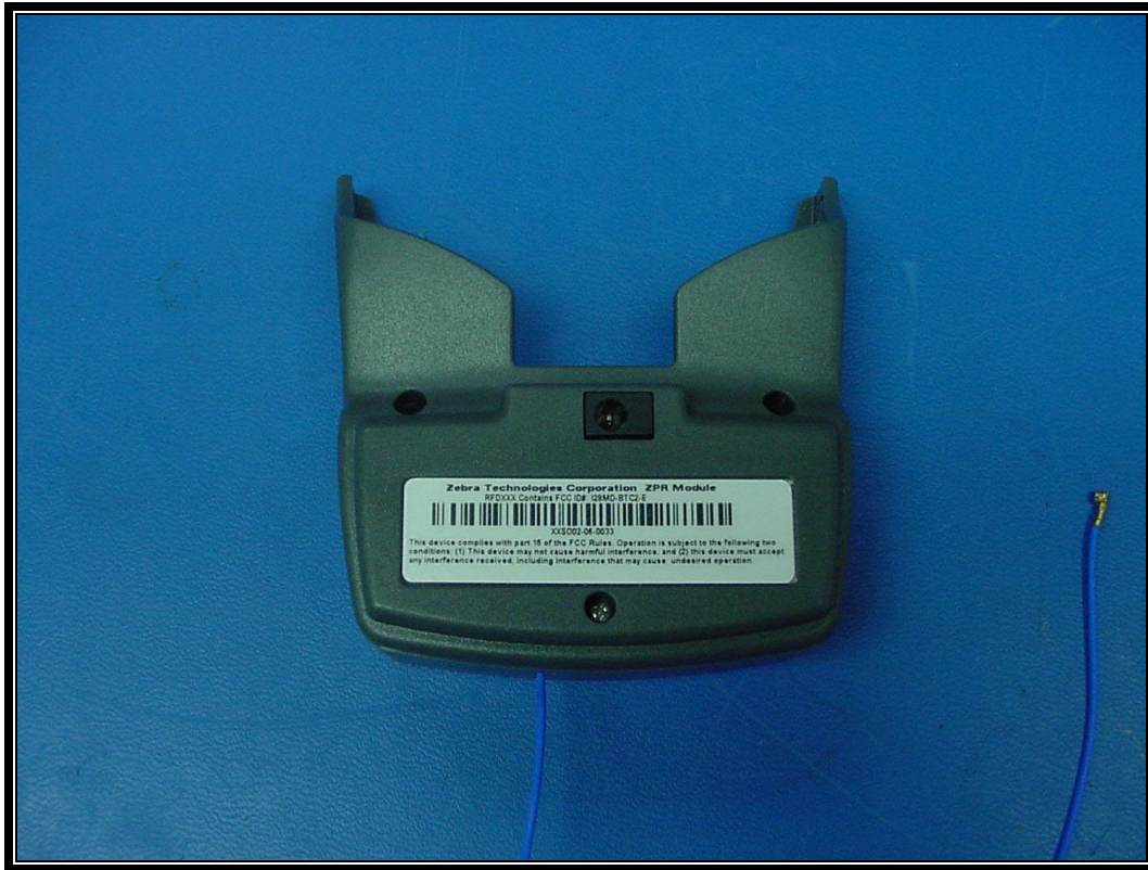
PHOTOGRAPH 27: REAR VIEW ZPR POD ANTENNA INSTALLED IN TYPICAL HOST
