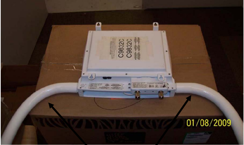
LAP-4200 External 2.4 GHz Antennas > 20 cm separation
