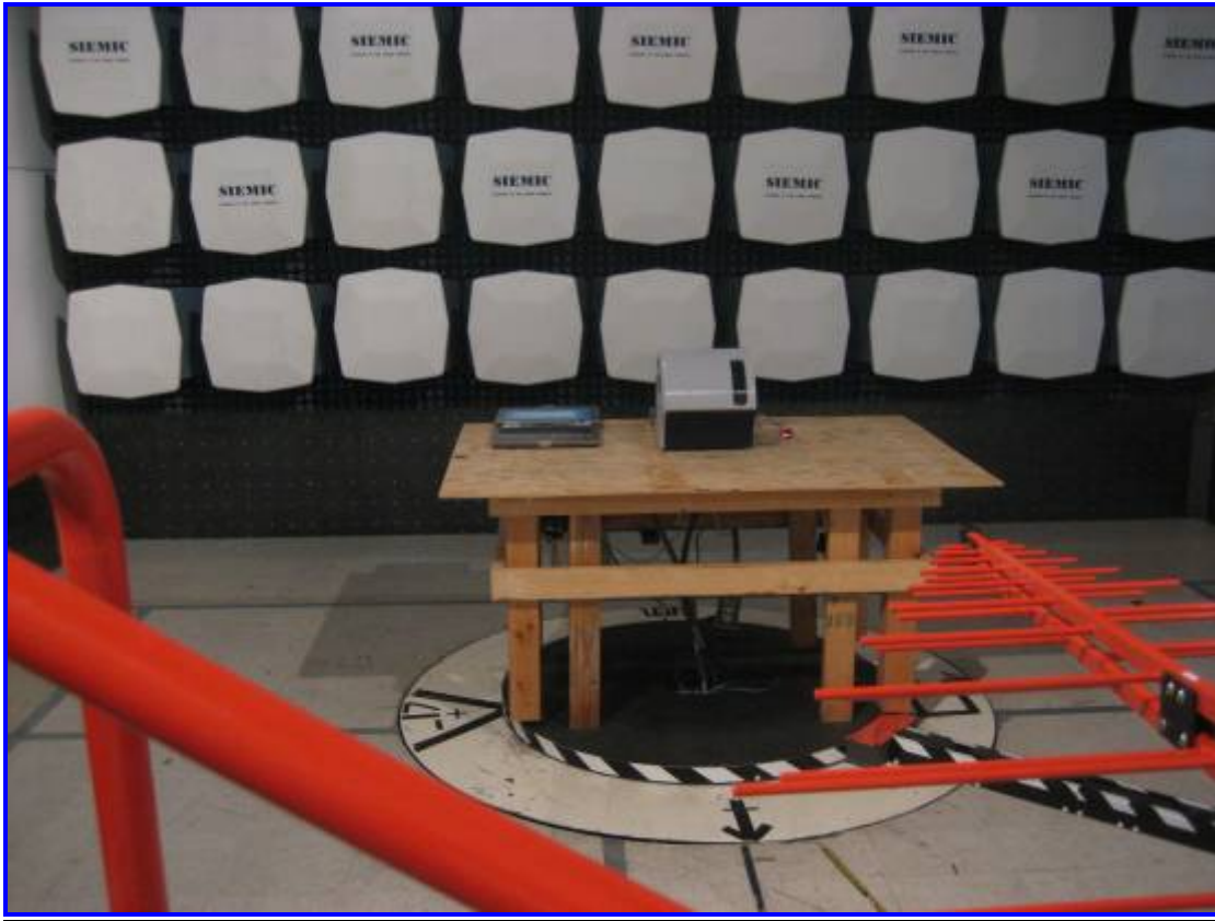
Radiated Emission Test Setup Front View (<1000MHz)
