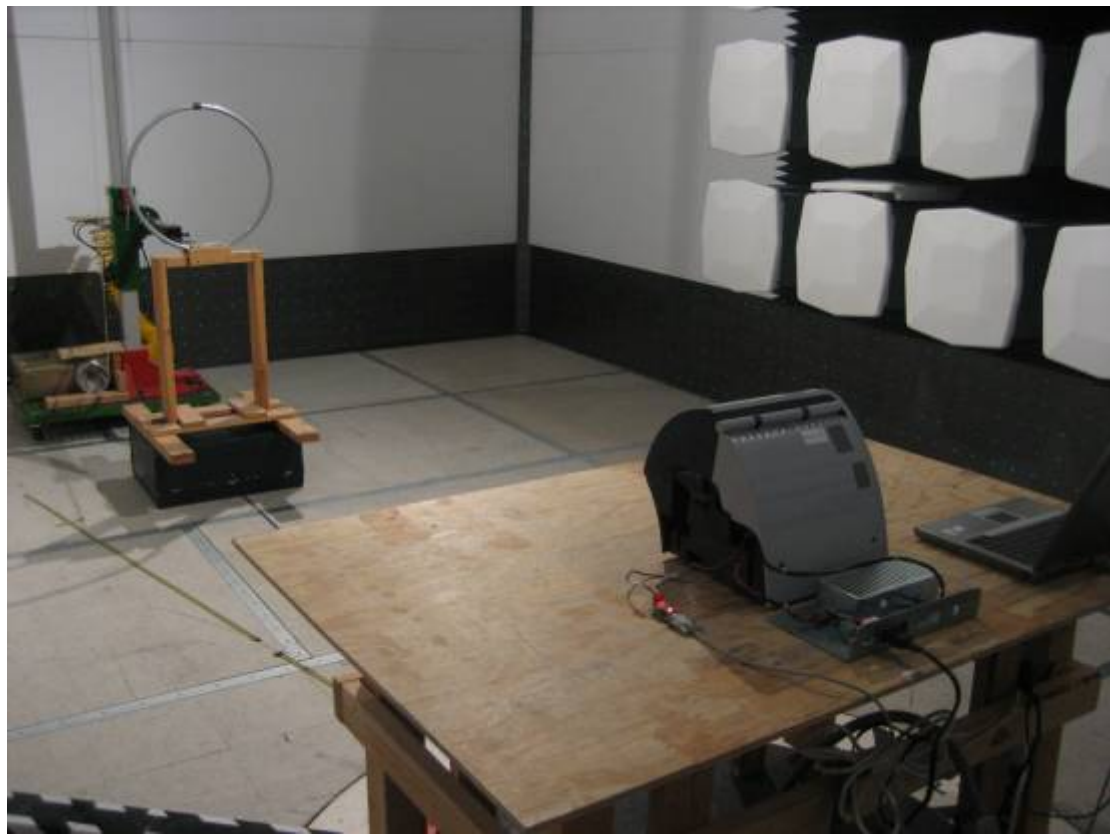
Radiated Emission Test Rear View (<30MHz)
