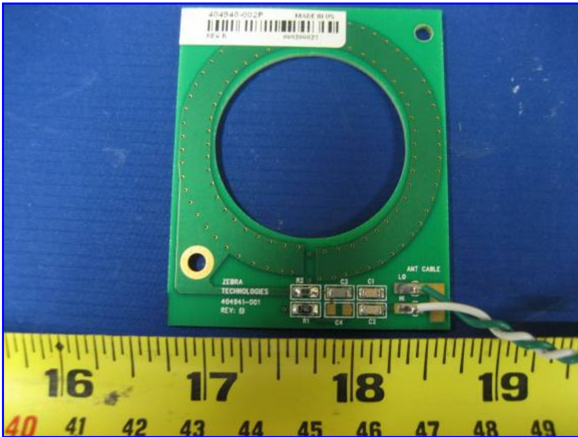
Antenna 2 (upper) Component View
