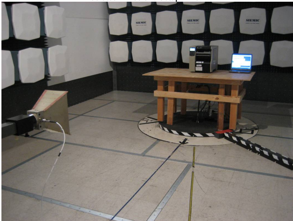
Radiated Emissions Setup - 140Xi4
