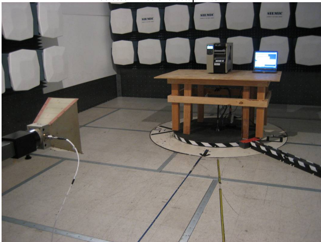
Radiated Emissions Setup - 140Xi4
