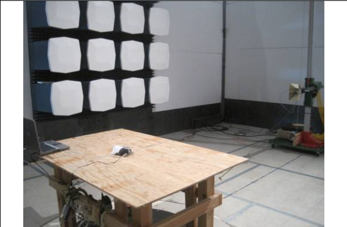
Radiated Emission Test Setup (above 1GHz) - Rear View
