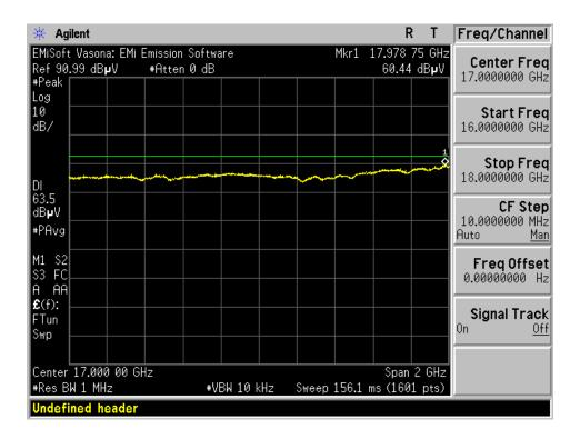
Note: above plot shows reduced VBW to make average measurements comparing to average limits and thus show compliance in range of 16-18GHz
