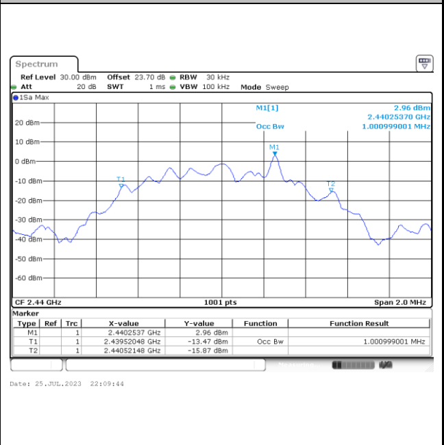
99% Occupied Plot Bandwidth on Channel 19
