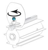
**6**. Slide the rewind media guide all the way out, and then fold it down.
