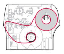
1. Extend the media approximately 18 in. (500 mm) out of the printer.
