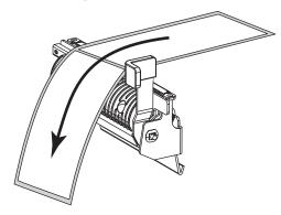
**3.** Thread the media into the slot below the peel assembly.
