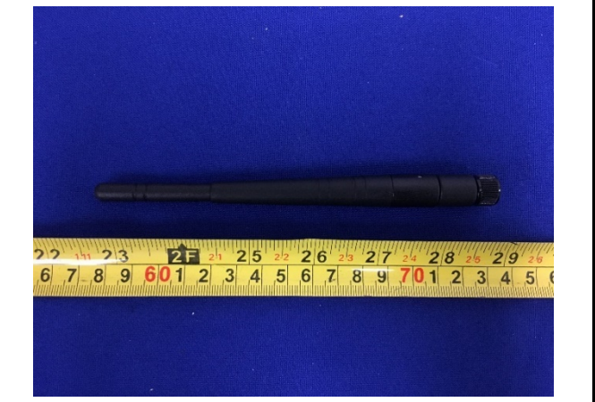
WLAN Antenna View
