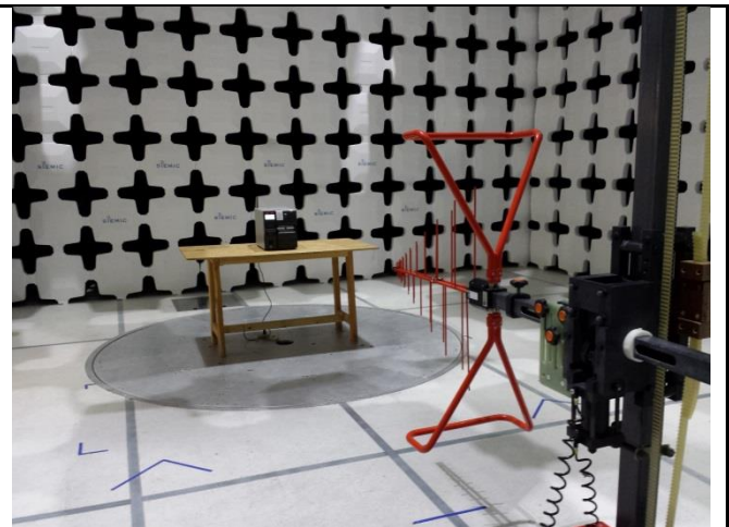
Radiated Emission below 1GHz – ZT410 (Rear)
