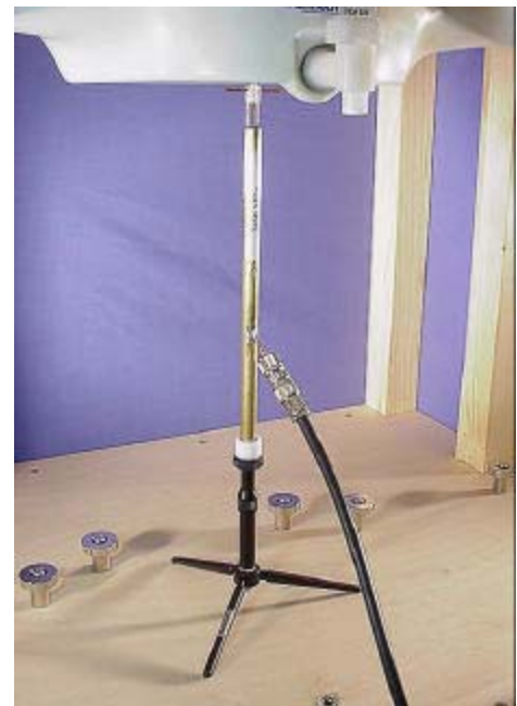
2450MHz System Check Setup Photograph
