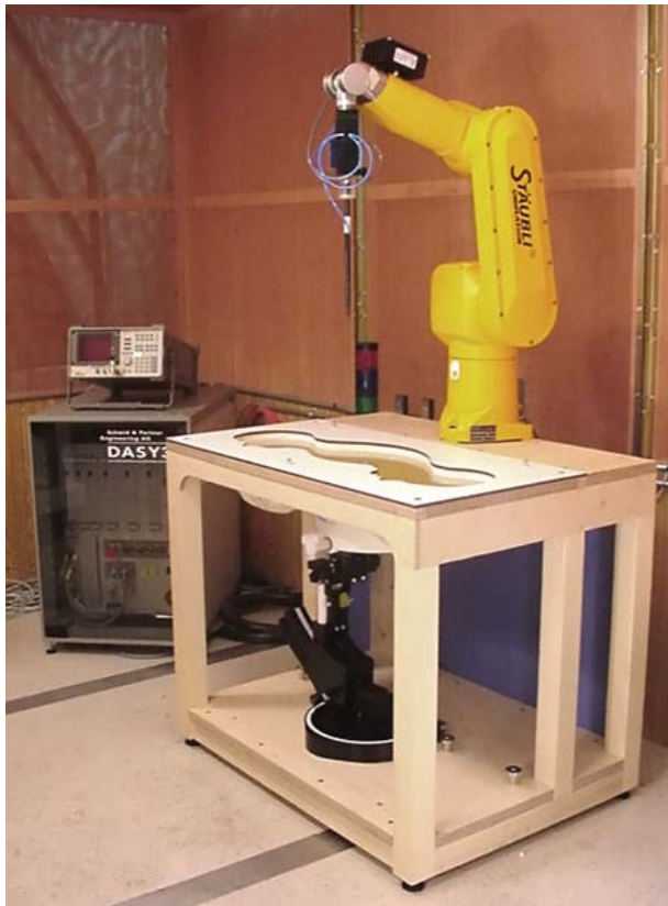
DASY3 SAR Measurement System with SAM phantom
