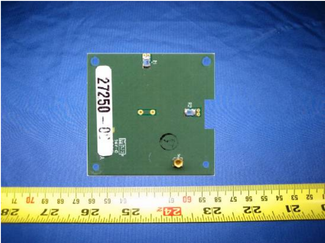
UHF Antenna Back View
