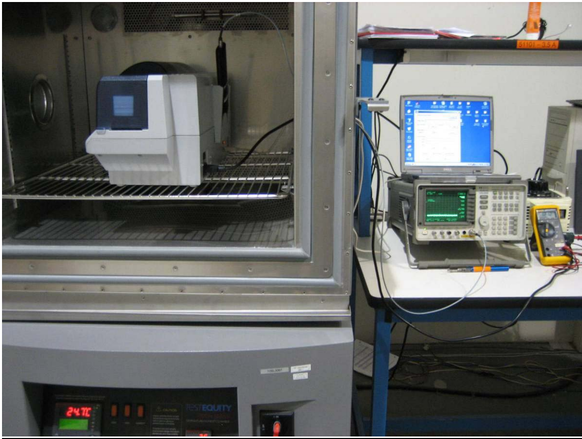
Frequency Stability test Setup View
