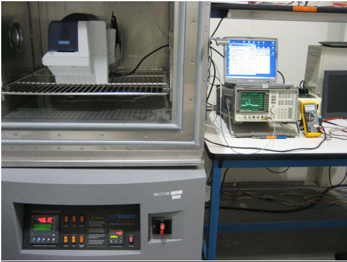
Frequency Stability Test Setup View
