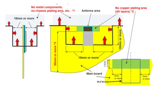
Note: a wide GND area must be provided to ensure isolation for each layer
