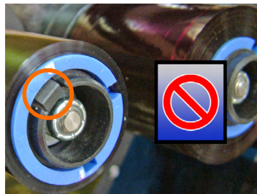
Wrong way: the core is not pushed fully against the back side, resulting in a Y border on the printed cards.
