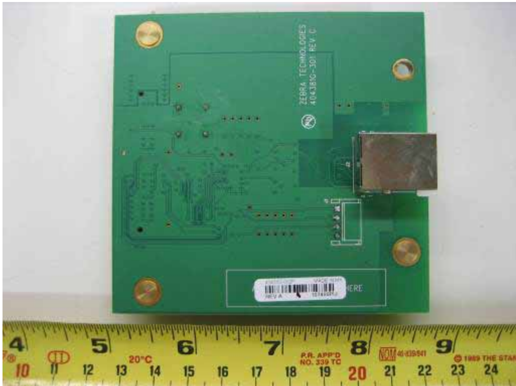
Ethernet Board- Bottom View
